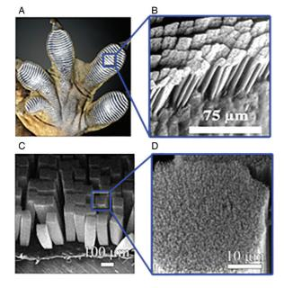
Figure 1: Gecko and synthetic setae. (A) Picture of a gecko foot showing the setae arranged into lobes on the foot. (B) Scanning electron microscope (SEM) image of gecko setae terminating into thousands of smaller spatulas (gripping hairs). Side view (C) and an SEM image (D) of synthetic setae. Image gratefully used with permission from Prof. Dhinojwala.<sup>1</sup> © National Academy of Sciences.
