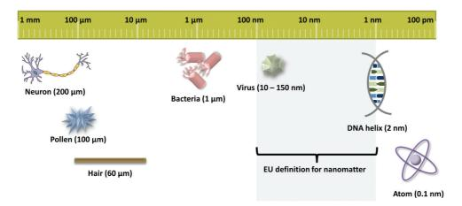
Figure 2: Explanatory scale of typical micro- and nano-sized objects. The EU defines nanomaterials as particles in the range of 1–100 nm.<sup>2</sup>
